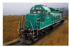
710ECO<sup>™</sup> Repowers extend locomotive life for up to 40 years and lower life cycle costs by equipping older models with EMD 710 engines. Benefits include lower emissions, 10 to 25% increase in fuel efficiency, 50% reduction in oil consumption, increased reliability, improved maintainability and enhanced diagnostics.
